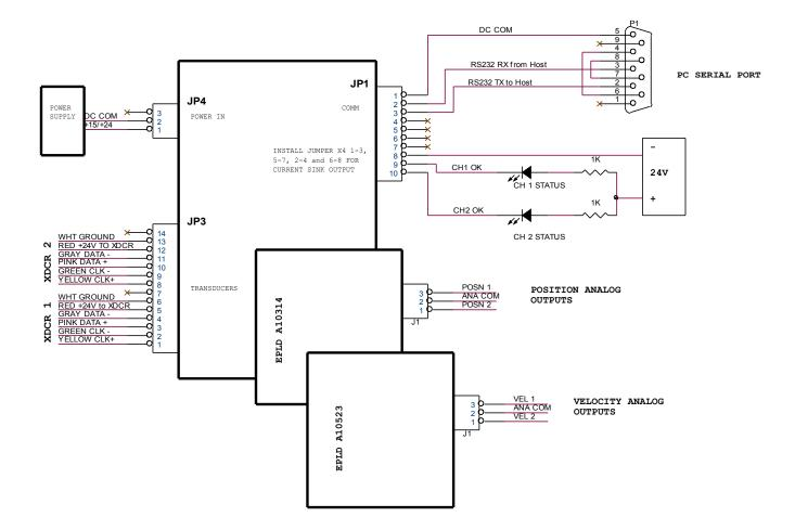
**Typical Connections 24V transducer**
